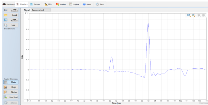
Figure 15 Terahertz signals from thick plastic coating on metal
